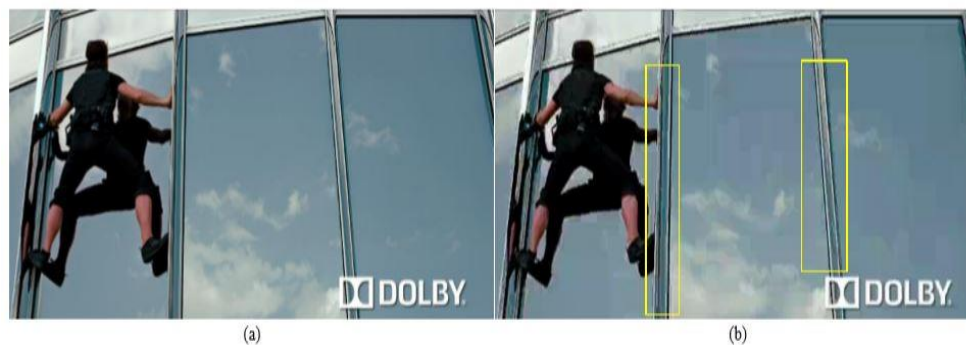
Figure 2. Ringing artifact (a) Reference frame; (b) Compressed frame with ringing artifact [9]
