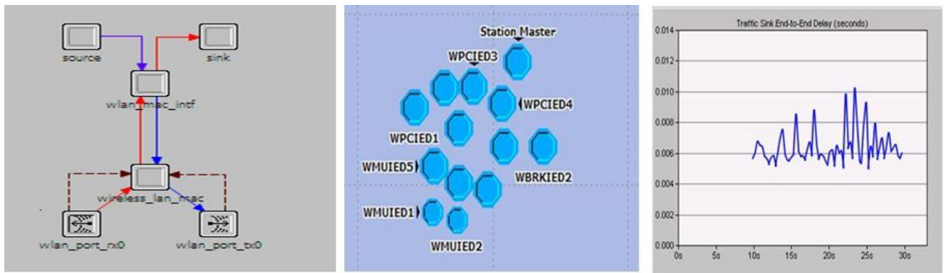
Figure 9. Node model diagram (left) for MUIED, wireless topology architecture (middle), and SV end-to-end delay measurement (right) for wireless topology architecture
