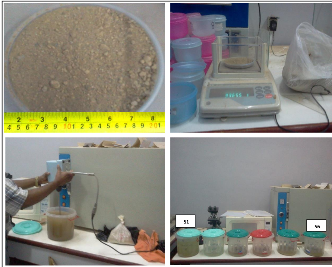
Figure 1. Phosphate rock material and leaching tank test procedure
