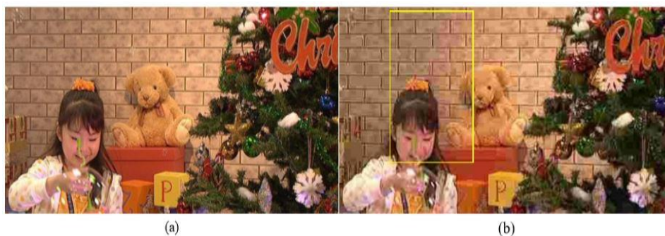
Figure 4. Color bleeding artifact (a) Reference frame (b) Compressed frame with color bleeding [10]
