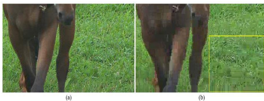
Figure 5: Basis image effect. (a) Reference frame (b) Compressed frame with basis pattern effect [9]
