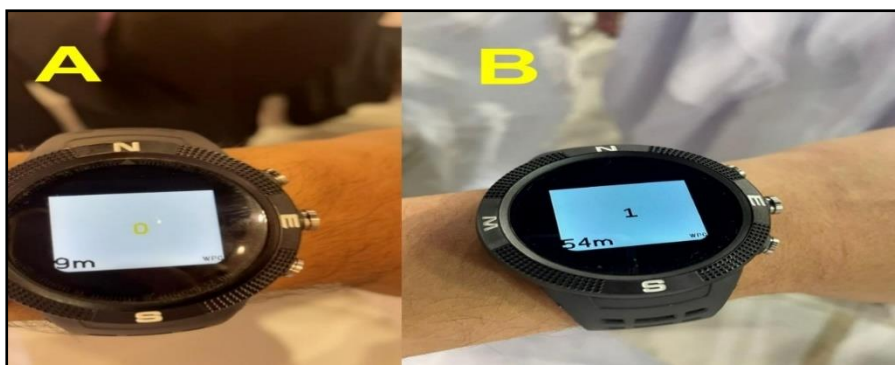
Figure 8. Screenshots of “Bangle.js” showing the Tawaf counter’s interface before and after a round.
