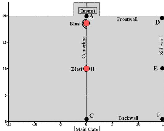
Fig. 1: Layout of the mosque showing the boundary conditions and assigned probe locations.
