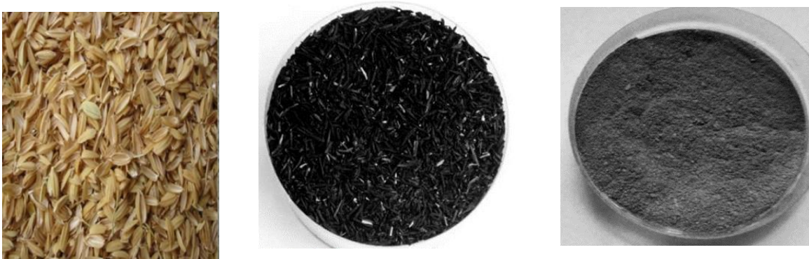
Fig. 1. a) Rice Husk [32], b) Burnt RHA [33] and c) burning of husk at about 700°C for 6 hours and wet grinding for 80 minutes [34]
