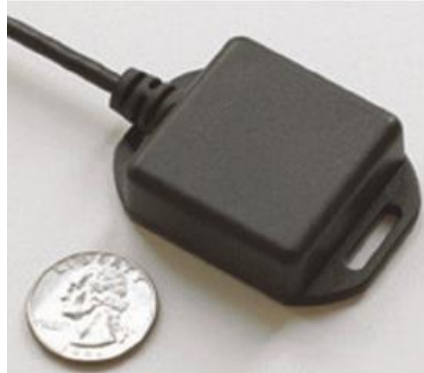
Figure 6. MotionNode device which includes an accelerometer, a gyroscope and a magnetometer.
